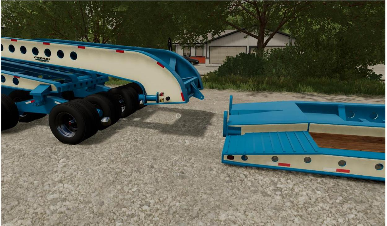
Put jeep and attached gooseneck onto trailer deck, then detach jeep and drive truck off.
