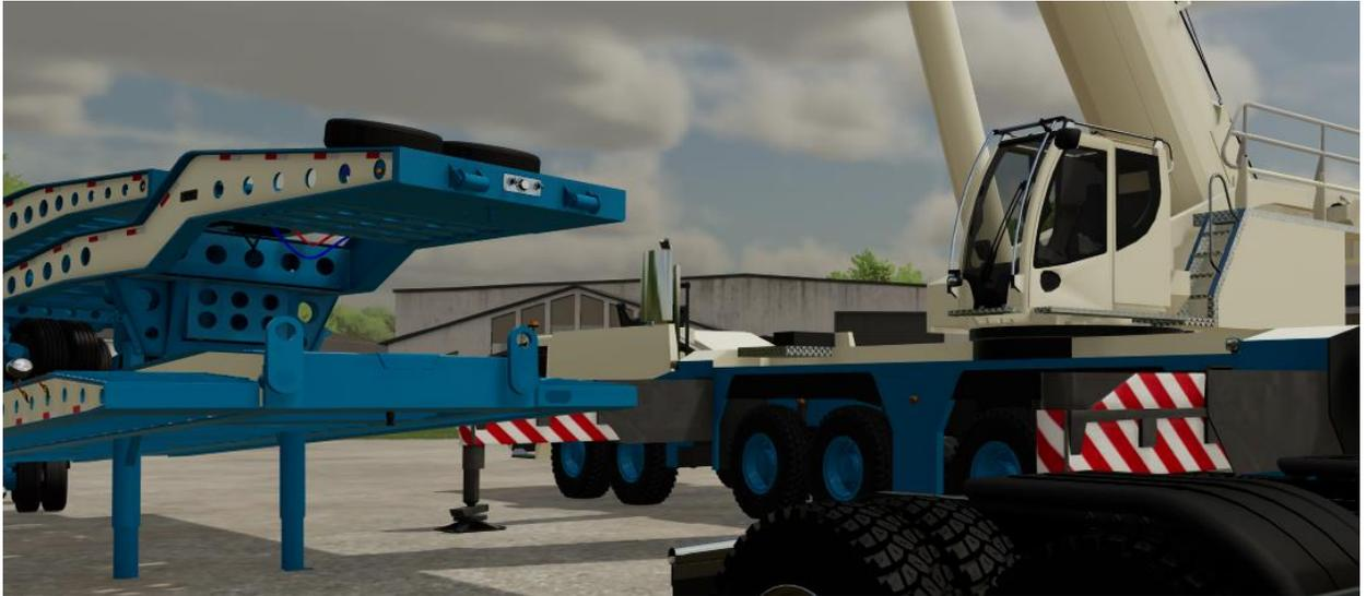
Drive truck under deck and attach. Raise supports.
